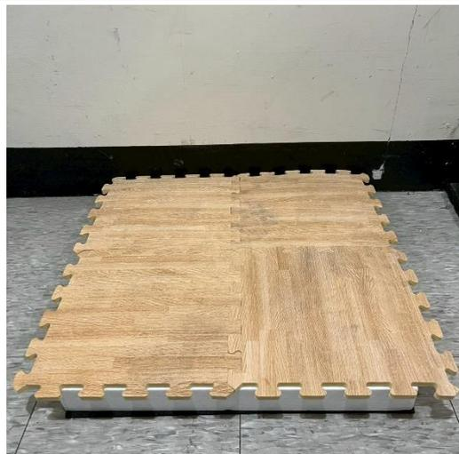
40mm EPS+5mm 橡膠隔音墊+10mm 巧拼
