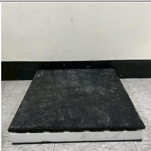
40mm EPS+5mm 橡膠隔音墊
