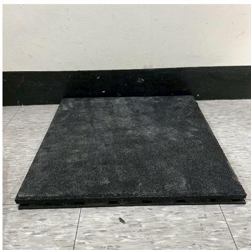
5mm 橡膠隔音墊+25mm 橡膠地磚
