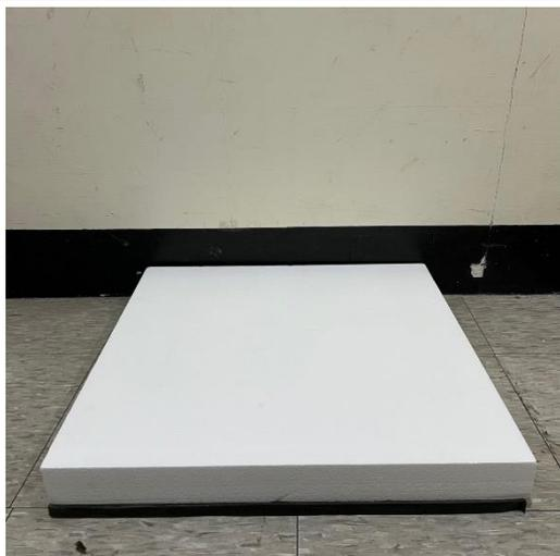
40mm EPS+15mm PE 隔音墊
